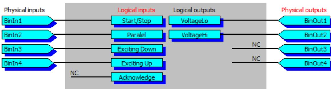
Having clicked on the name of the logical input (Logical inputs) or physical output (Physical outputs) in the Mapping window (I/O Mapp) of the service program Manager there will appear the window for selection where the signal in question is to be connected.
