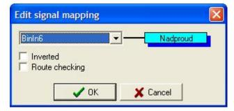
It is possible to connect the signal also inverted (Inverted) and if it is available for HW it is possible at input to activate the route checking (Route checking).
