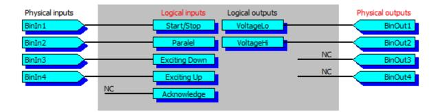
Having clicked on the name of the logical input (Logical inputs) or physical output (Physical outputs) in the Mapping window (I/O Mapp) of the service program Manager there will appear the window for selection where the signal in question is to be connected.
