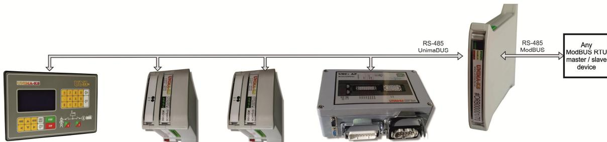
The bridge can read information from several control systems connected to the UnimaBUS bus and then provide it on the ModBUS bus under one common ModBUS address. In this case, all control systems must have a different UnimaBUS address set on the UnimaBUS.
