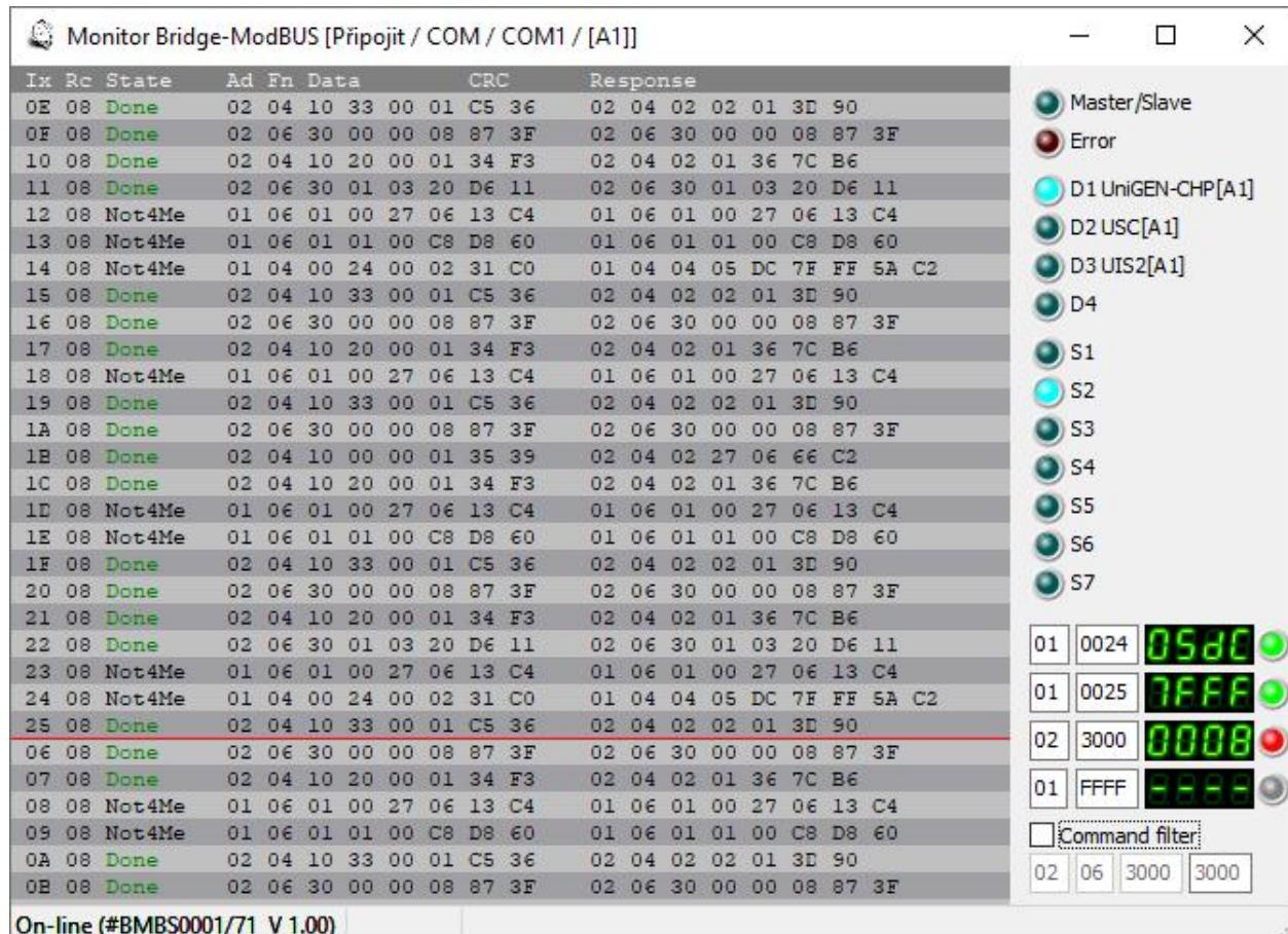
ModBUS communication (question and answer) is displayed in the monitor. In slave mode, queries for other devices on the ModBUS bus (devices with an address other than Bridge) are also displayed, including the answers of these devices (label "Not4Me"). In the event of a fault, a label with an error code is displayed.
