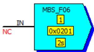
Command for writing the value connected to the block input to the device register 0x0201 at address 1, sent periodically every two seconds.
