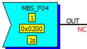
Command to read register 0x0200 from device at address 1, sent periodically every second. The read value is stored in the quantity connected to the block output (User analog output). The user analog outputs can then be used in mapping in any device on the UnimaBUS bus, similarly to banks W and X. In this way, a maximum of 16 analog values can be read (UsrBO01-UsrBO16).
